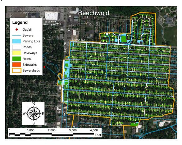
Figure 25. Map showing impervious surface types in the Beechwold sewershed. Pervious areas in the sewershed are not highlighted with color.
