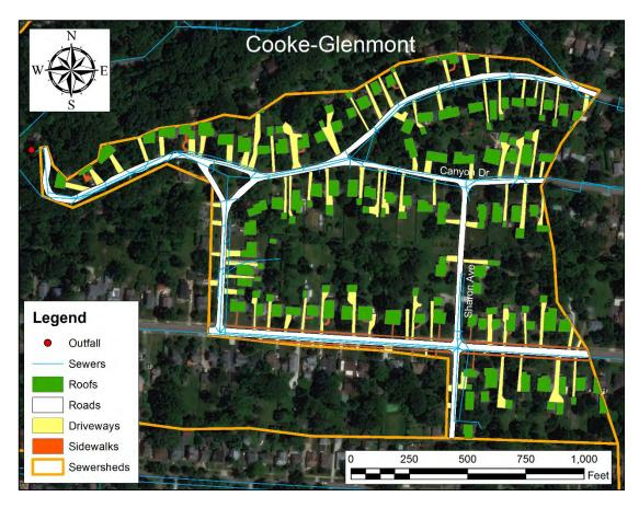
Figure 27. Map showing impervious surface types in the Cooke-Glenmont sewershed. Pervious areas in the sewershed are not highlighted with color.
