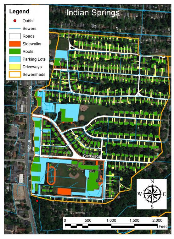
Figure 26. Map showing impervious surface types in the Indian Springs sewershed. Pervious areas in the sewershed are not highlighted with color.
