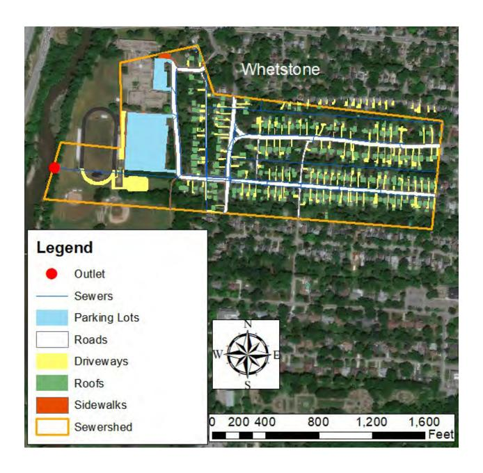
Figure 30. Map showing impervious surface types in the Whetstone sewershed. Pervious areas in the sewershed are not highlighted with color.
