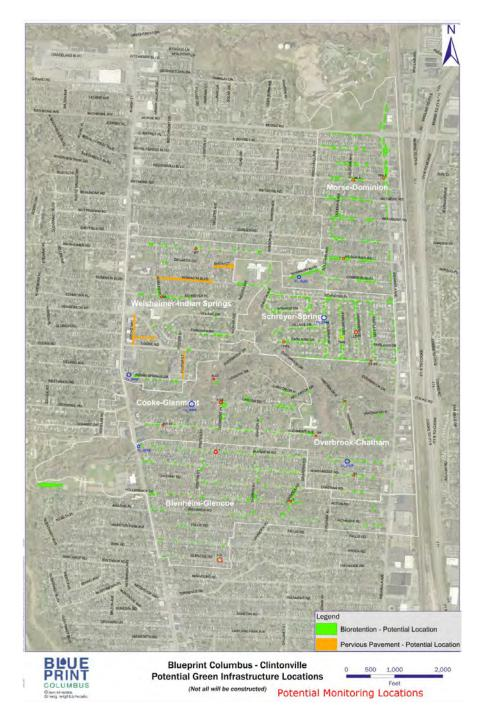
Figure 24. Locations of bioretention (green) and permeable pavement (orange) retrofits planned for the Clintonville neighborhood. The areas of Clintonville being monitored are outlined in blue (control sewershed) and white (green infrastructure retrofits).
