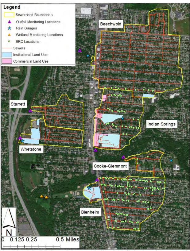
Figure 2. Boundaries of the six sewersheds monitored in this study. Distribution of green infrastructure (GI), monitoring locations, and land use within each sewershed also shown. Remaining area within each sewershed not identified as Commercial or Institutional is Residential land use.
