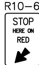
The sign post should be centered on the stop line and placed as close as possible to 3 ft. behind the curb or 6 ft. off of the edge of pavement.
