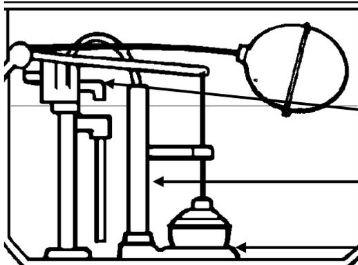
If the **refill valve** is not working properly, it does not shut off the refill water at the proper time. Water fills the tank until it reaches the opening to the **overflow pipe**, then it silently runs down the overflow pipe into the bowl and out the main drain. An average refill valve leak consumes about 1 / 2 gallon per minute.
