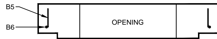
SECTION E COLLAR - REBAR INSTALLATION
