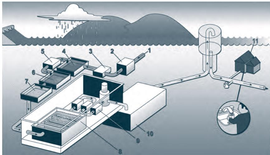
Water flows (1) to the treatment plant from the reservoir or stream through rotating screens (2) to remove large debris. It is then pumped into the plant where alum is added (3) to cause coagulation. After rapid mixing, the water remains in the settling basin (4) while sedimentation of floc occurs (2-4 hours). The water treatment residual (settled floc) is pumped from the bottom of the pools and stored in holding lagoons to dry.
