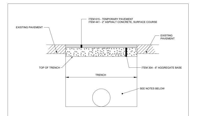
BACKFILL FOR ALL TRENCHES SHALL BE IN ACCORDANCE WITH APPLICABLE SPECIFICATIONS.
