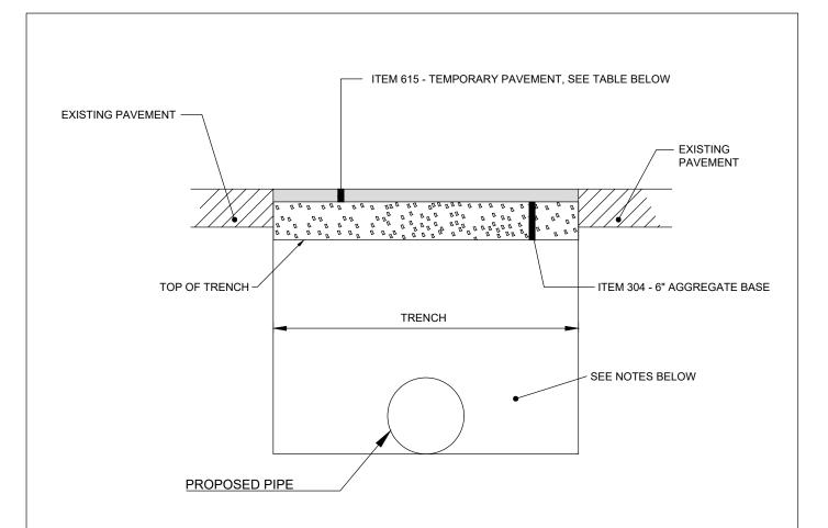
BACKFILL FOR ALL TRENCHES SHALL BE IN ACCORDANCE WITH APPLICABLE SPECIFICATIONS.
