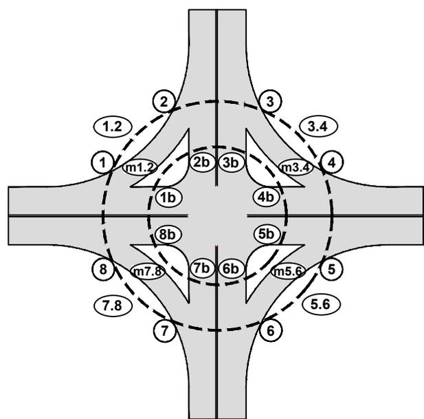
ALL NUMBERING BEGINS FROM THE NORTHWEST CORNER AND GOES CLOCKWISE. EACH CORNER HAS ITS SPECIFIC NUMBER THAT SHALL BE USED IF CURB RAMPS ARE IN THESE LOCATIONS.
