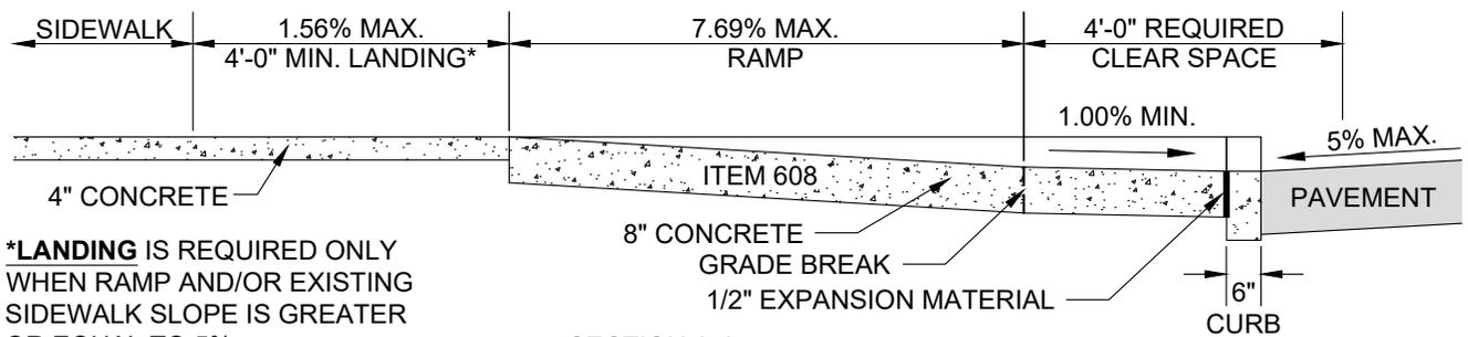
\*LANDING IS REQUIRED ONLY WHEN RAMP AND/OR EXISTING SIDEWALK SLOPE IS GREATER OR EQUAL TO 5%
