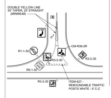
THE DESIGN SHOWN IS REFERENCED TO A WB-50 TURNING TEMPLATE AS AN EXAMPLE ONLY. THE DESIGNER SHALL PROVIDE THE DIMENSIONAL REQUIREMENTS FOR THE MAXIMUM SIZE DESIGN VEHICLE REQUIRED FOR THE SITE.
