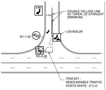
THE DESIGN SHOWN IS REFERENCED TO A WB-50 TURNING TEMPLATE AS AN EXAMPLE ONLY. THE DESIGNER SHALL PROVIDE THE DIMENSIONAL REQUIREMENTS FOR THE MAXIMUM SIZE DESIGN VEHICLE REQUIRED FOR THE SITE.
