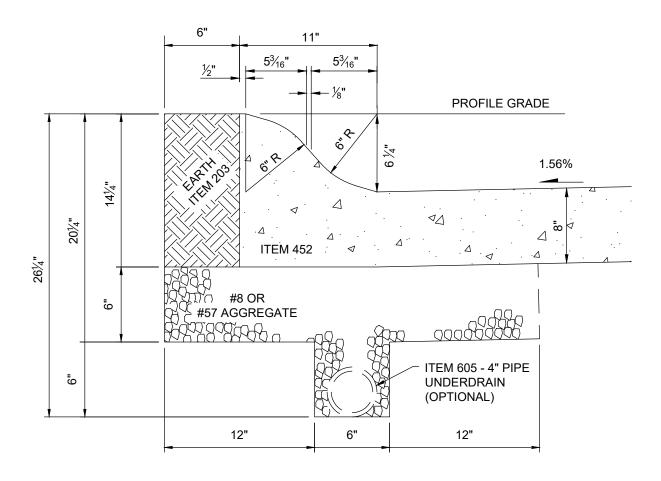
ITEM 452 - 8" NON-REINFORCED CONCRETE PAVEMENT WITH INTEGRAL CURB
