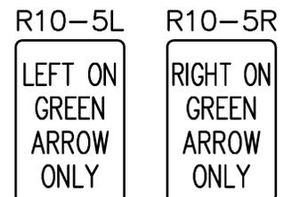
The Right On Green Arrow Only sign (R10-5R, 30 in. x 36 in.) shall be used where traffic signal heads control exclusive right turn movements (protected
