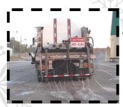
Anti-icing is the proactive application of melting products to driving surfaces before a winter weather event. Anti-icing helps prevent snow and ice from bonding to the
