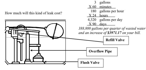
If the <u>refill valve</u> is not working properly, it does not shut off the refill water at the proper time. Water fills the tank until it reaches the opening to the **overflow pipe**, then it silently runs down the overflow pipe into the bowl and out the main drain. An average refill valve leak consumes about 1 / 2 gallon per minute.
