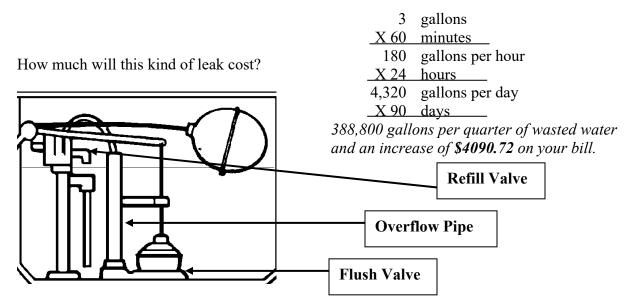
If the <u>refill valve</u> is not working properly, it does not shut off the refill water at the proper time. Water fills the tank until it reaches the opening to the **overflow pipe**, then it silently runs down the overflow pipe into the bowl and out the main drain. An average refill valve leak consumes about 1 / 2 gallon per minute.
