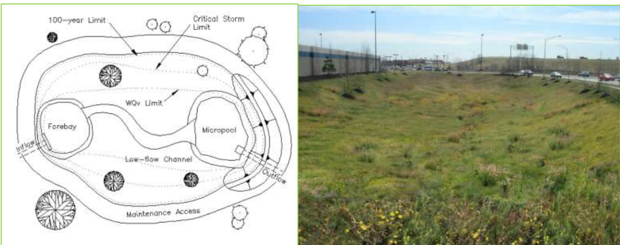
FIGURE 4-1 PLAN VIEW OF DRY DETENTION BASIN DESIGN (LEFT) AND TYPICAL DRY DETENTION POND (RIGHT)
