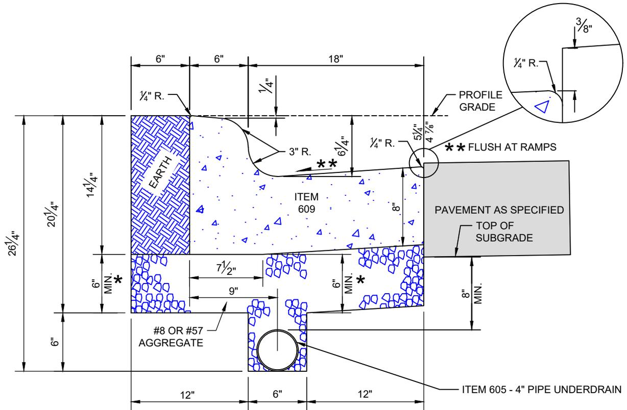
\* CURB AND GUTTER AGGREGATE COURSE-WHERE THE ROADWAY PAVEMENT HAS AGGREGATE BASE, MATCH THE BOTTOM OF THE CURB AND GUTTER AGGREGATE COURSE TO THE TOP OF SUBGRADE. ENSURE ROADWAY SUB BASE MEETS UNDERDRAIN AGGREGATE.
