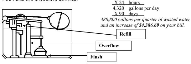
If the <u>refill valve</u> is not working properly, it does not shut off the refill water at the proper time. Water fills the tank until it reaches the opening to the **overflow pipe**, then it silently runs down the overflow pipe into the bowl and out the main drain. An average refill valve leak consumes about 1/2 gallon per minute.
