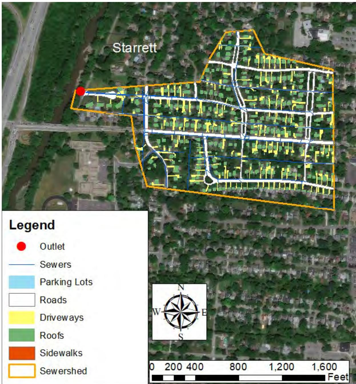
Figure 29. Map showing impervious surface types in the Starrett sewershed. Pervious areas in the sewershed are not highlighted with color.
