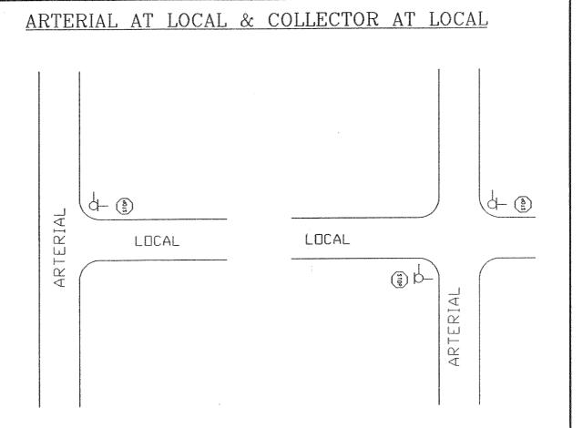
ALL SIGNS SHALL BE 12" HIGH x REQUIRED LENGTH, MOUNTED 14' ABOVE GROUND. SIGNS SHALL BE LOCATED FAR RIGHT FOR THE ARTERIAL WITH TWO SIGNS PER POST. IF THE COMBINED SQUARE FOOTAGE OF THE TWO SIGNS EXCEEDS 10 SQ. FT. USE SEPERATE POST FOR EACH SIGN AS ABOVE.
