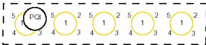
**Figure A PQI Measurement Pattern**
