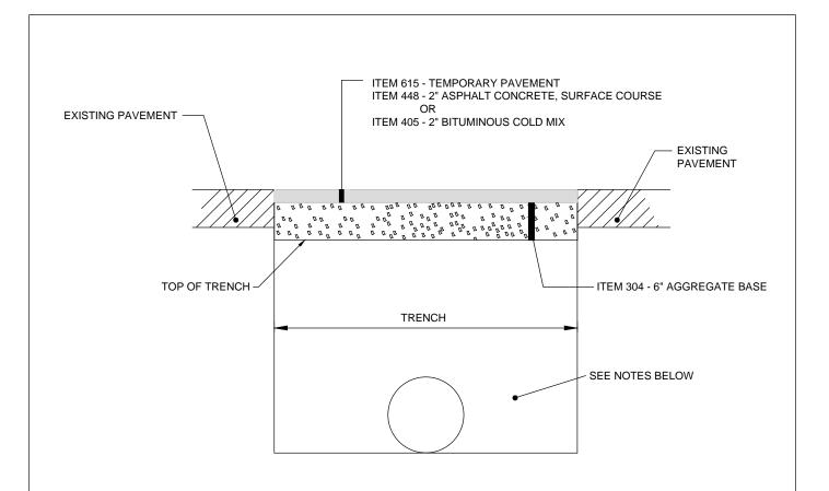
BACKFILL OF ALL TRENCHES SHALL BE IN ACCORDANCE WITH APPLICABLE SPECIFICATIONS.
