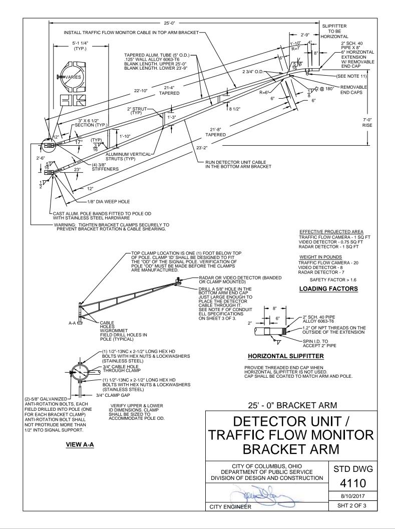
INSTALL THE TRAFFIC FLOW MONITOR CABLE IN THE TOP ARM BRACKET. INSTALL THE DETECTOR CABLE IN THE BOTTOM ARM BRACKET.
