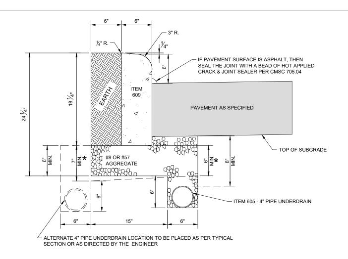
\* CURB AGGREGATE COURSE-WHERE THE ROADWAY PAVEMENT HAS AGGREGATE BASE, MATCH THE BOTTOM OF THE CURB AGGREGATE COURSE TO THE TOP OF SUBGRADE. ENSURE ROADWAY SUB BASE MEETS UNDERDRAIN AGGREGATE.
