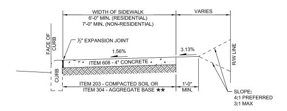
WHERE SIDEWALKS ABUT DRIVEWAYS OR ALLEY APPROACHES, THE CONCRETE THICKNESS OF THE WALK SHALL EQUAL THE THICKNESS OF THE APPROACH (6" MINIMUM) FOR A DISTANCE OF ONE (1) FULL PANEL OR MINIMUM 5 FEET. SEE STANDARD DRAWING OF THE APPLICABLE DRIVEWAY OR ALLEY.
