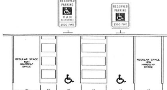
SIGNS SHALL BE MOUNTED AT A MINIMUM OF 7' FROM GROUND TO BOTTOM OF SIGN
