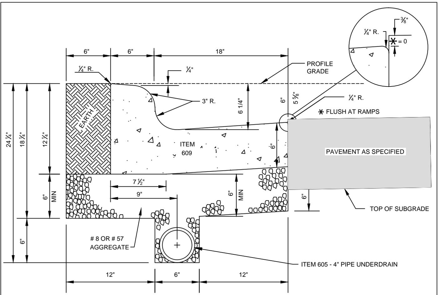
\* THE PAVEMENT SHALL BE FLUSH AT THE GUTTER IN FRONT OF CURB RAMPS. CURB RAMPS SHALL BE BUILT PER STD DWG 2319.
