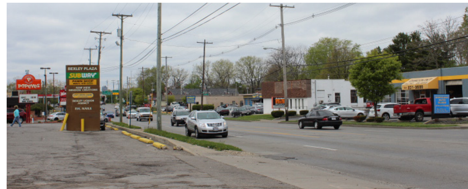
Multiple curb cuts along the commercial section of Livingston Ave
