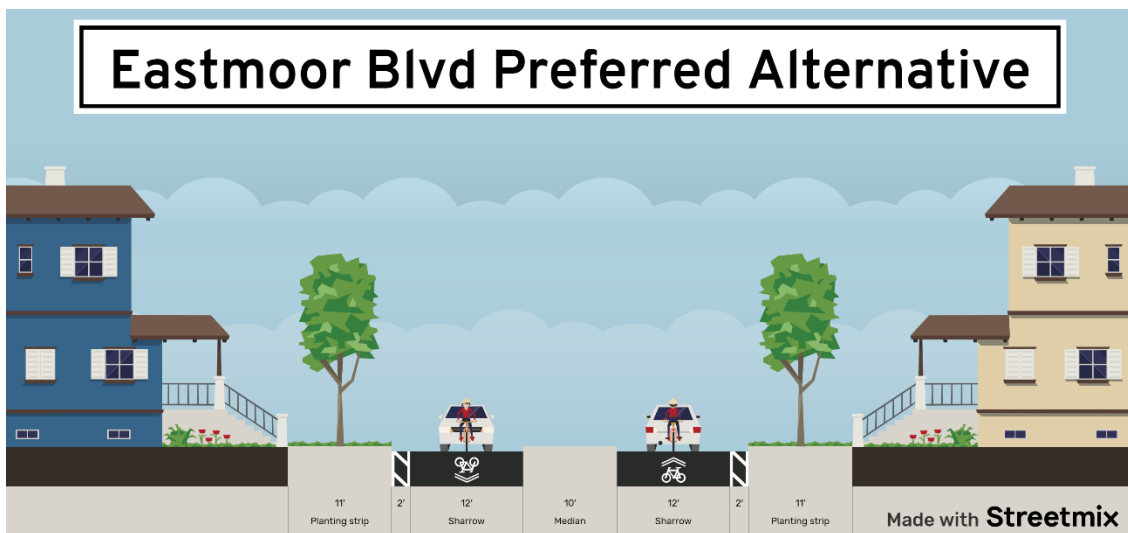
Figure 6. Cross Section of Preferred Alternative – Median
