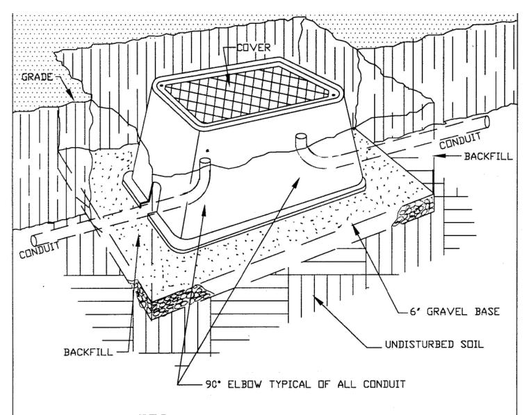
NOTES: THE BACKFILL SHALL BE POWER TAMPED IN LAYERS NOT EXCEEDING 4 INCHES IN THICKNESS LODSE MEASUREMENTS COMPLYING WITH SOIL DENSITY COMPACTION REQUIREMENTS UNDER SECTION 203.12 OF THE CIY OF COLUMBUS CONSTRUCTION AND MATERIAL SPECIFICATIONS.
