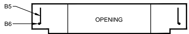
SECTION E COLLAR - REBAR INSTALLATION
