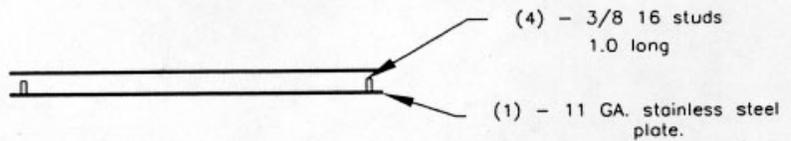
STAINLESS STEEL HARDWARE SHALL BE SUPPLIED FOR FASTENING OF ENCLOSURE.
