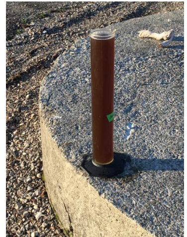
Leachate is very turbid and generally similar to raw sewage except higher in ammonia and nitrogen.
