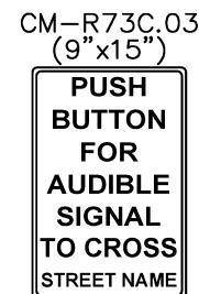
Figure 6.4 Audible Pushbutton Sign
