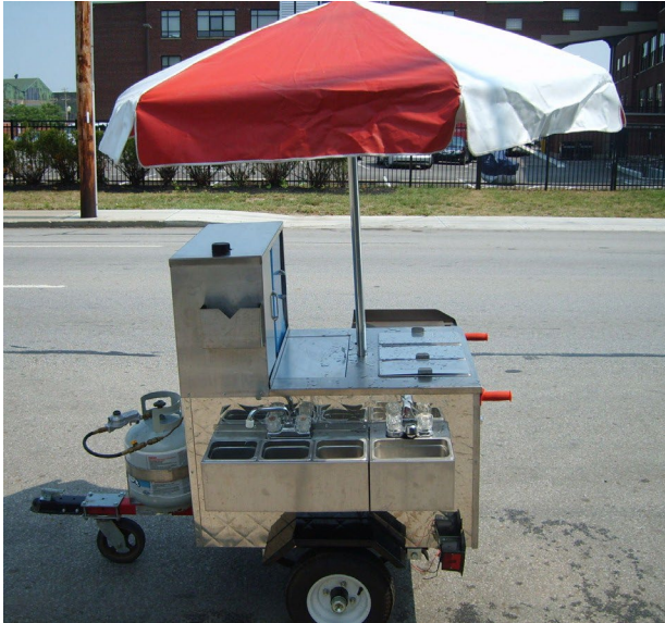
An example of a pushcart with a three compartment sink and a handsink.
