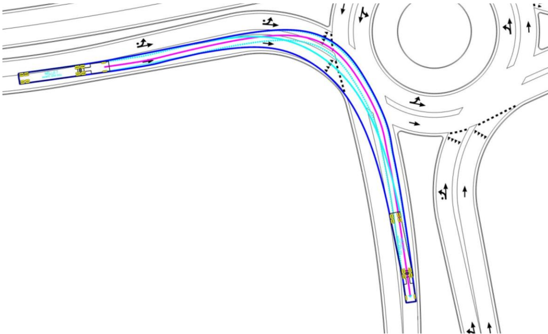
Figure 36 – Straddle Lanes Design: Right Turn Movement
