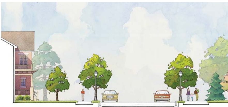
A typical parkside neighborhood street section showing parking on one side of a two-way street and deeper lot setbacks to accommodate outdoor living and to respond to open space addresses
