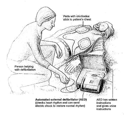
The image shows a typical setup using an automated external defibrillator (AED). The AED has step-by-step instructions and voice prompts that enable an untrained bystander to correctly use the machine.
