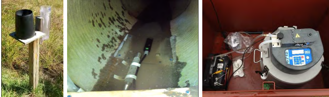
Figure 2. Rain gage setup (left), sample intake (clear plastic) and area velocity meter (black) in the Cooke-Glenmont outfall (center), and automated sampler at Beechwold (right).
