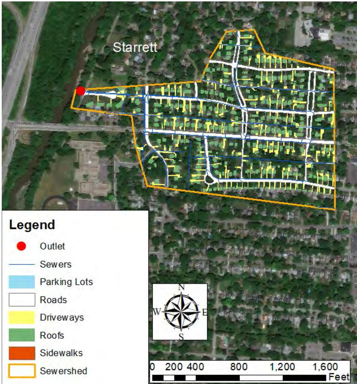
Figure 31. Map showing impervious surface types in the Starrett sewershed. Pervious areas in the sewershed are not highlighted with color.
